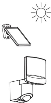
It is recommended to put the solar panel in the sun for 8 hours to charge the battery.
